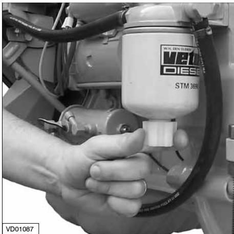
Empty fuel filter
