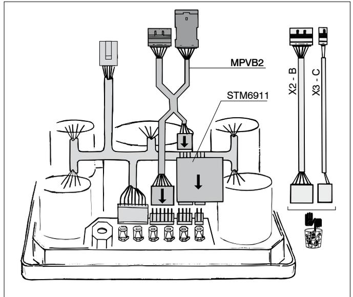
Install interface pcb [STM6911] onto warning light pcb. Connect Interface cable [MPVB2] to warning light pcb and to interface pcb.
