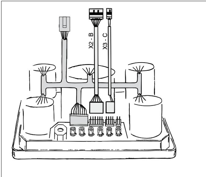
On panel, remove connection cables, X2 ↔ B and X3 ↔ C, from warning light printed circuit board (pcb).
