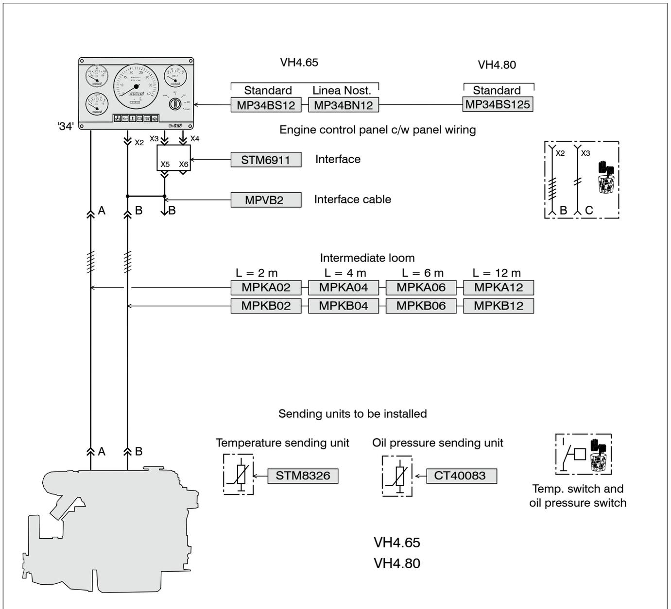
When using a panel model '34' both warning lights and meters, for coolant temperature and oil pressure have to be operated.
