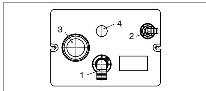
If more supply connections are required drill extra holes (ø 43 mm, 1 11/16" dia.) for the extra fittings.
