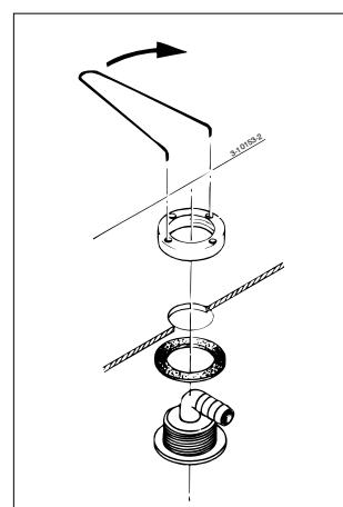
To prevent blockages caused by hairs and coarse waste in particular, all fittings should have burrs removed internally, local narrowing should be reduced to a minimum and any changes in pipe diameter should be done using conical adapters or large radii.
