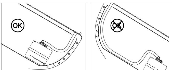
When fitting remember that the filler hose must always be positioned on the same side of the ship as the tank.
