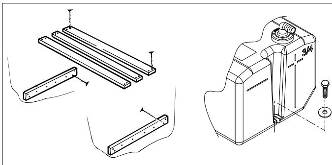
Ensure that there is a sufficiently solid foundation for placing and fixing the tank firmly.
